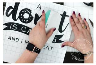
Use a scrapper or brayer over the transfer tape to ensure the top vinyl surface is properly adhered.
